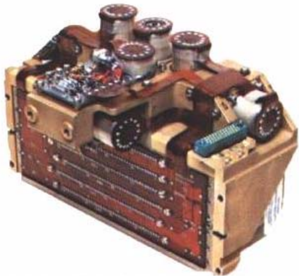
Same unit, using a 16 Layer flexible circuit.
